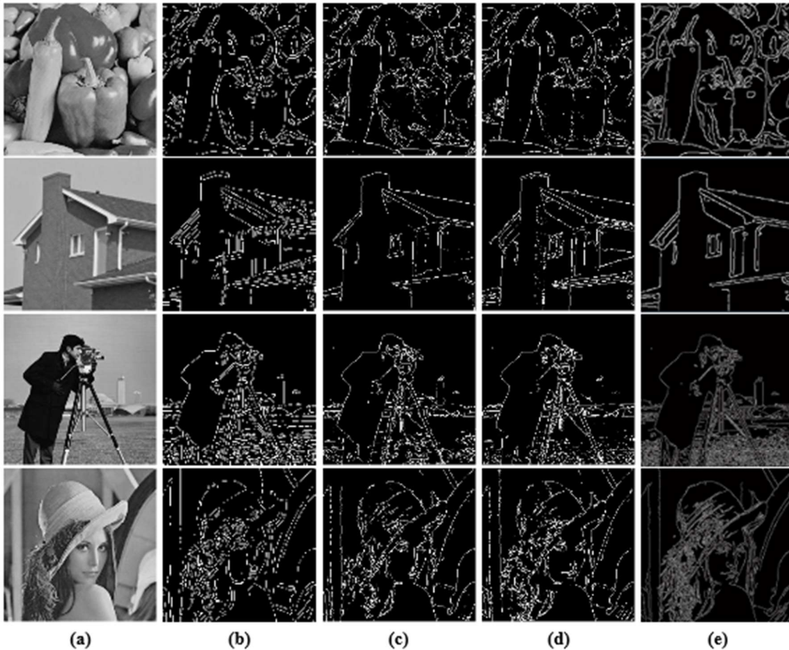
Fig. 1. Test Results of Standard Images Edge Detection (a) Original Image (b) Canny Operator (c) Log (d) FCMACO (e) ACPSO
