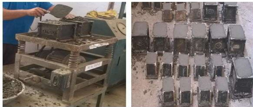
Figure 1: Casting of Cube Specimens
