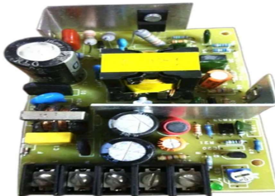
Fig 1: 12 V CCTV SMPS Power Supply interior view
