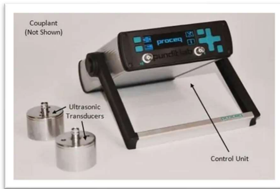
Fig 3. UPV Test Machine Working
