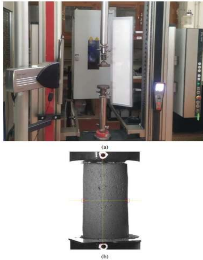
Fig.4: (a) Uniaxial Compression Test Setup with Video Extensometer System, (b) Gauge Point Detection in the Video Extensometer System
