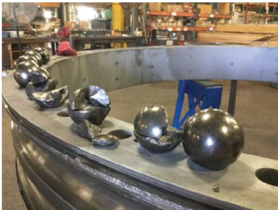
(c) Fractured balls
