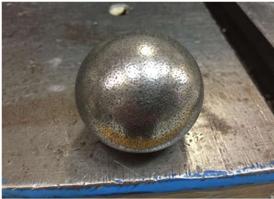
(a) Corrosion pitting in ball
