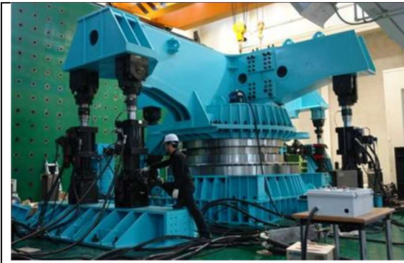
Fig 13: Pitch bearing test rig [42]
