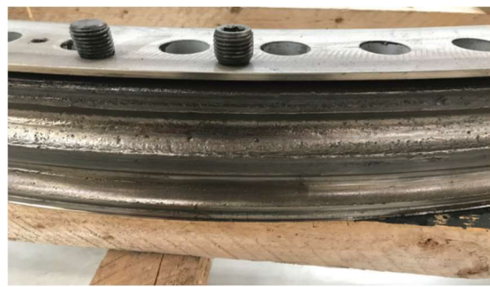
(b) Core crushing and cold working
