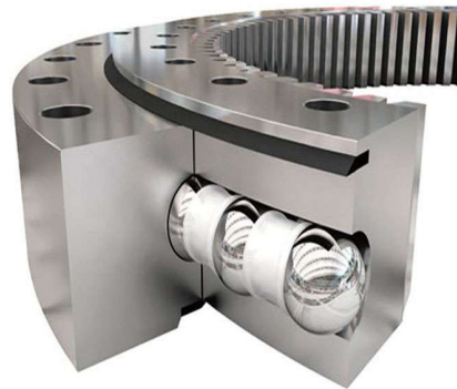
Fig 4. Cut section Four-point contact ball bearings single-row slewing bearing with internal gears [7]
