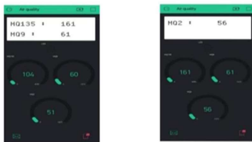
Figure 6: Air ranges of MQ2, MQ9, MQ135
